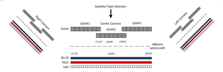
Observations are taken at resolutions between 100 and 180 m at nadir up to 350 and 660 m at the swath extremes for the VNIR and SWIR channels, respectively (*Francois et al, 2014*)
