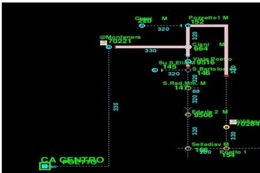
RETIM Replay allows to calculate the new value of AV20 managing the network once the feeder is repowered. In this case the value of AV20 (min\*customers) is 15.18. This evaluation means that introducing a rational network management, a potential SAIDI reduction is possible. Furthermore it is interesting to highlight that by the use of this test method it is possible to measure the KPI identified as SRI (SAIDI Reduction Index).<sup>7</sup>
