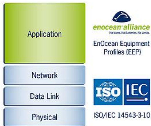
Figuur 3-20 de protocol stack ISO/IEC 14543-3-10 (bron EnOcean)
